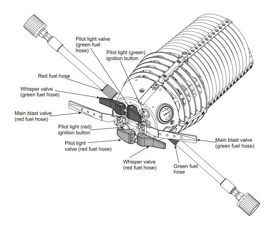
The outer dimensions, positions of the support rods' sockets and the carabiners' attachment points of the BASIC and SIRIUS burner frame are the same, therefore the BASIC and SIRIUS burner frames are interchangeable.
