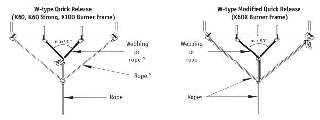
ouse quick release set with red ropes when attaching to the burner frame use quick release set with green ropes when attaching to the basket lugs
