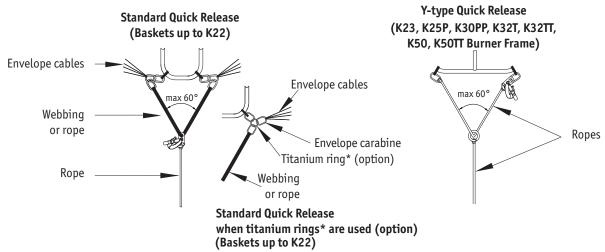
\*if titanium rings are used, they have to be fitted at all attachement points
